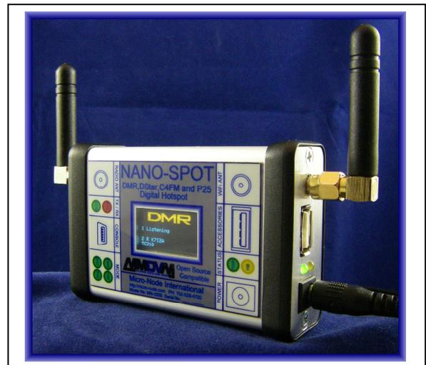
The built-in USB Type Mini B console port allows access to the Linux Operating system for advanced users when WiFi network access is unavailable.
